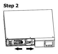
Disconnect battery wires.
