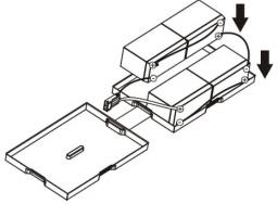
**6-battery kit** Step 1: Remove adhesive tapes.
