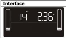
SettingParameter 2: Set up the charger boost voltage.2.25-2.40: setting the charger boost voltage from 2.25V/cell to 2.40V/cell. (Default: 2.36V/cell)
